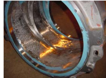
Inside of body after cladding
